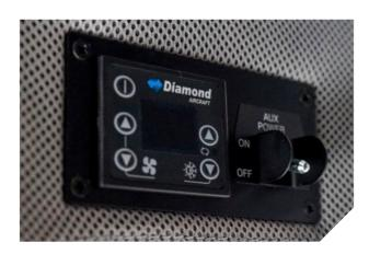
Air conditioning/RACC II system (powered by an additional alternator)
