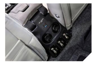
USB power outlets for pilot & co-pilot and passengers in the 2<sup>nd</sup> row Dual headset plugs (LEMO connector + standard jack connector)
