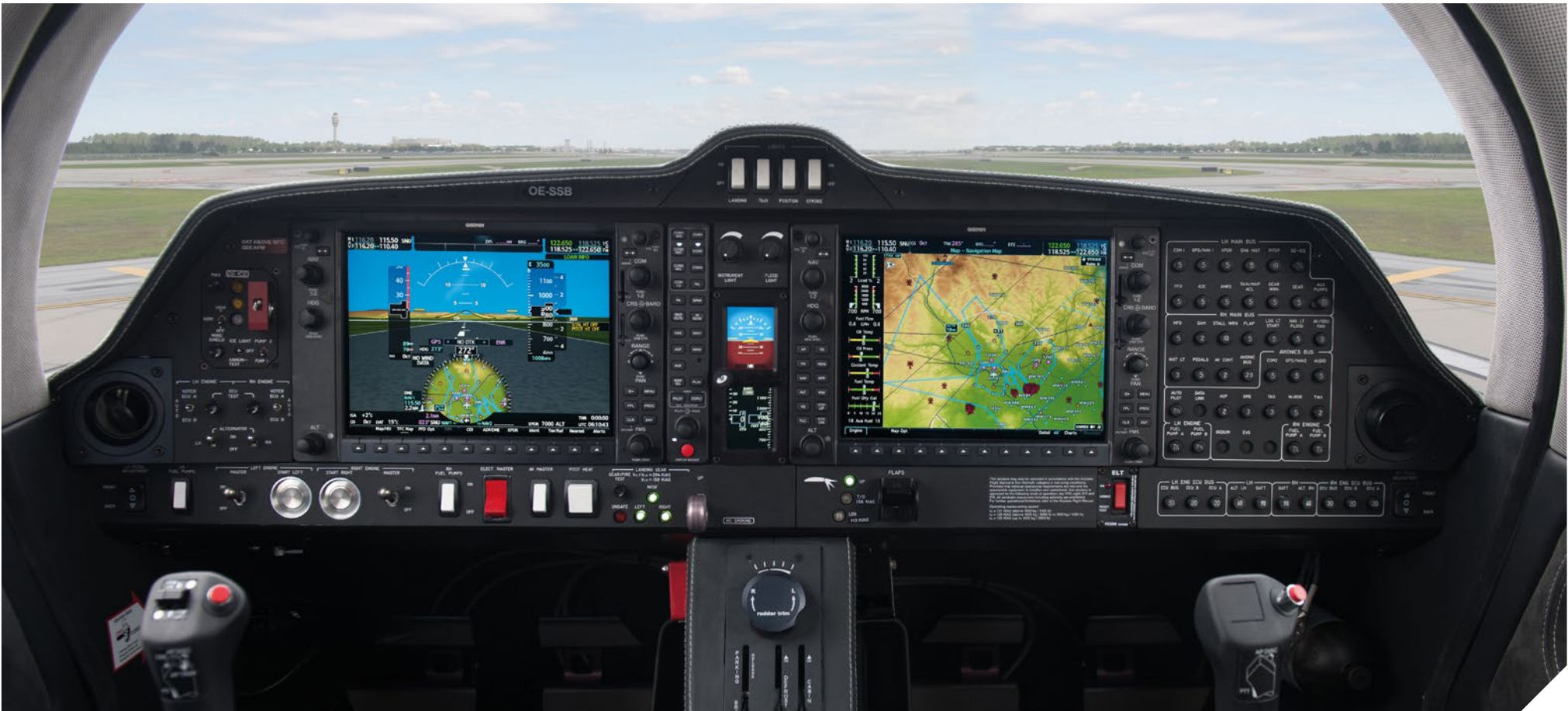
Integrated Garmin G1000 NXi glass panel cockpit
