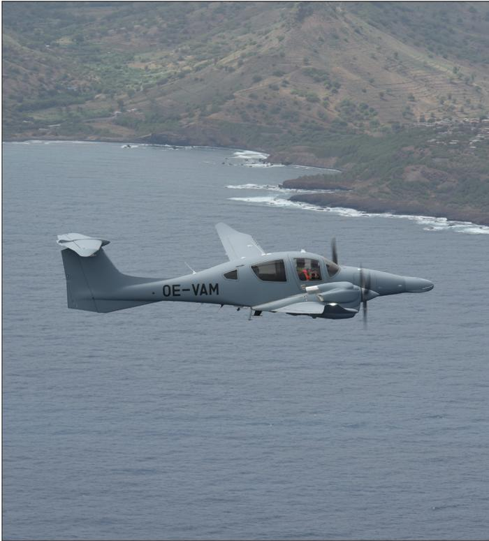
The DA42 MPP PANDION is a cost-effective maritime patrol turnkey solution, featuring two in-house designed components, the light weight maritime search radar NEPTUN and the commercial satellite communication system KOPERNIKUS, and an electro-
